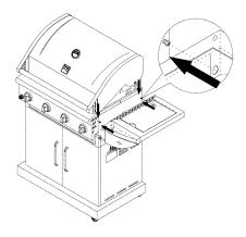
4. Using (2)  $1/4 \times 10$ mm screws and (2) 1/4 lock washers, attach side burner shelf to grill head from inside the firebox. Do not tighten screws.
